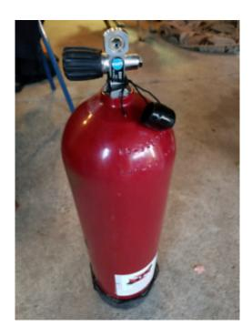
A diving cylinder, scuba tank or diving tank is a gas cylinder used to store and transport the high pressure breathing gas required by a scuba set. It may also be used for surface-supplied diving or as decompression gas or an emergency gas supply for surface supplied diving or scuba. Cylinders provide gas to the diver through the demand valve of a diving regulator or the breathing loop of a diving rebreather.
